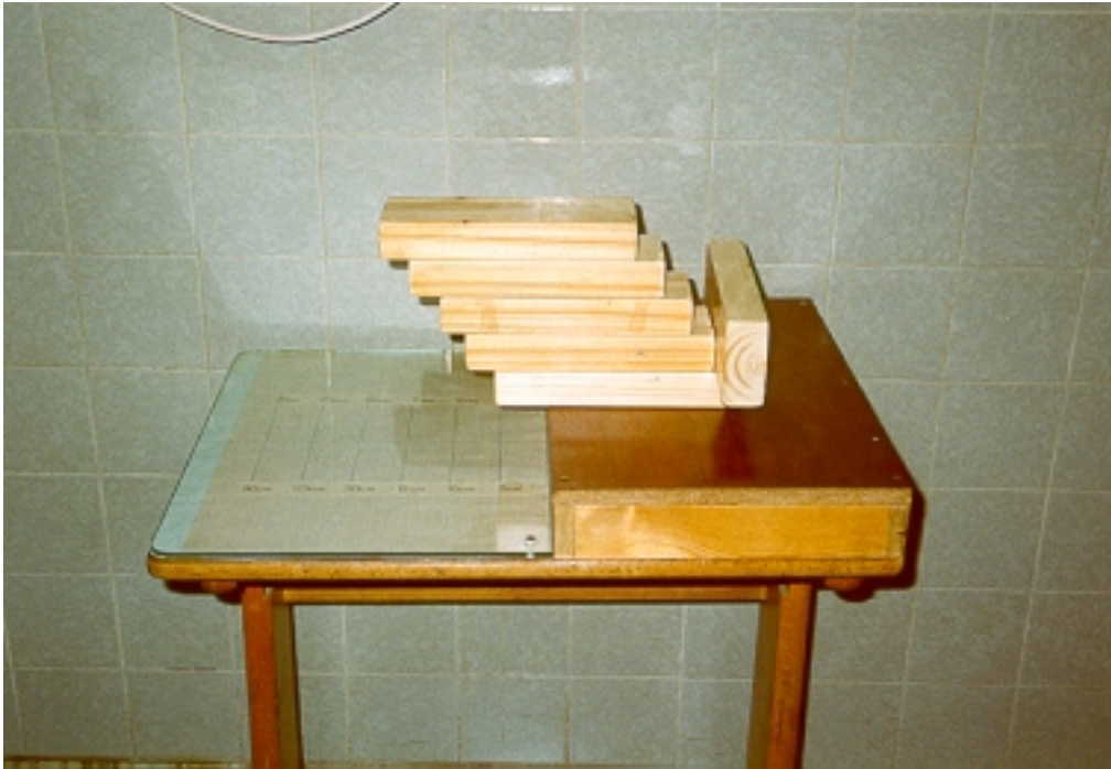
Fig. 3: With the given square wooden blocks a “slanted tower”, which is jutting from the edge as far as possible without collapsing, is meant to be built. Its width is being measured and put down on a list.
