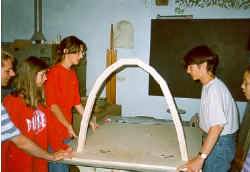
Fig. 1: Students cooperate to build a new experiment station to be set up in the school's corridor: when building a bridge with bricks which are shaped like the line of a chain turned upside down, the bridge remains stable even without "glue". At the Hardenberg-Gymnasium the experiments you can touch have become a popular pastime during the breaks.
